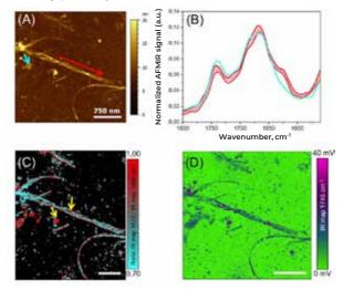
a) O-PTIR image of the neuron acquired at 1650 cm<sup>-1</sup> (proteins) (b) OPTIR spectra. Scalebar 20  $\mu$ m. c) AFM image of the same primary neuron. D) OPTIR signal from the neuron cell body to the cell neurite
