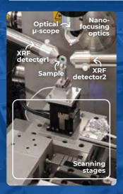
Scanning multi-length scale imaging with spatial resolution readily adaptable in the 100 nanometer - 1 micron range is provided routinely. This multilength scale "zoom-in" capability is well adapted to the study of complex heterogeneous samples and of tinv features embedded in intact mesoscale samples.
