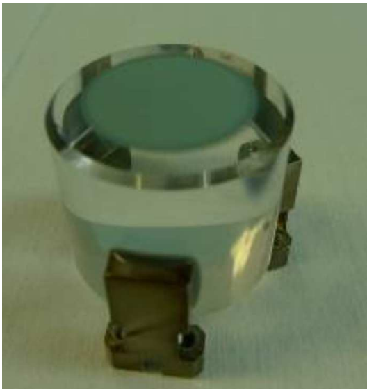
Fig. 3. Picture of the HRI EUV secondary mirror flight model before integration in the EUI instrument.
