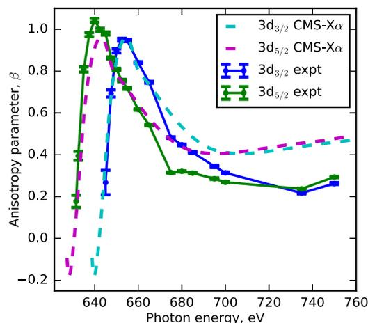
FIG. 8. The experimentally derived photoelectron anisotropy parameters for the I  $3d_{5/2}$  (green) and I  $3d_{3/2}$  (blue) levels in  $\text{CH}_3\text{I}$ . The error bars represent the standard error of the  $\beta$  parameters extracted from the fit. The corresponding theoretical (CMS- $X\alpha$ ) photoelectron anisotropy parameters are plotted for the I  $3d_{5/2}$  (magenta) and I  $3d_{3/2}$  (cyan) levels using the experimental ionization energies.
