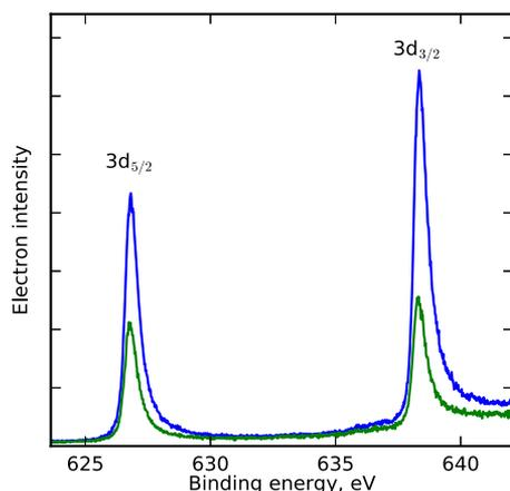
FIG. 7. Photoelectron spectrum of  $\text{CH}_3\text{I}$ , recorded at a photon energy of 665.6 eV, using parallel (blue) and perpendicular (green) linearly polarized radiation. The two bands are due to ionization of the I  $3d_{5/2}$  and I  $3d_{3/2}$  levels. The asymmetric band shapes are the result of post collision interaction.
