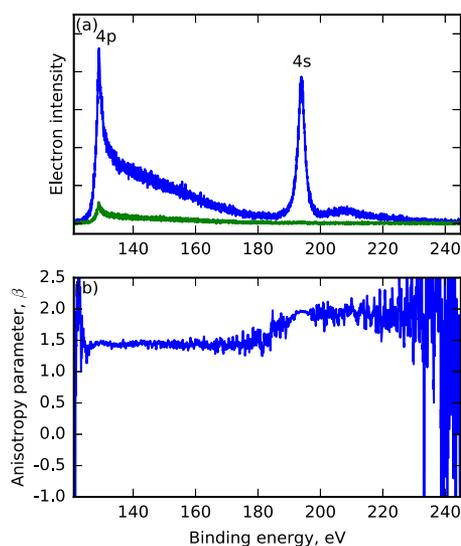
FIG. 6. (a) Photoelectron spectrum of  $CH_3I$ , recorded at a photon energy of 614.0 eV, using parallel (blue) and perpendicular (green) linearly polarized radiation, in the binding energy range encompassing structure due to the  $I\ 4s$  and  $I\ 4p$  orbitals. (b) The corresponding photoelectron anisotropy parameter. A 10-point moving average has been applied to the anisotropy parameter spectrum to improve the signal-to-noise ratio.
