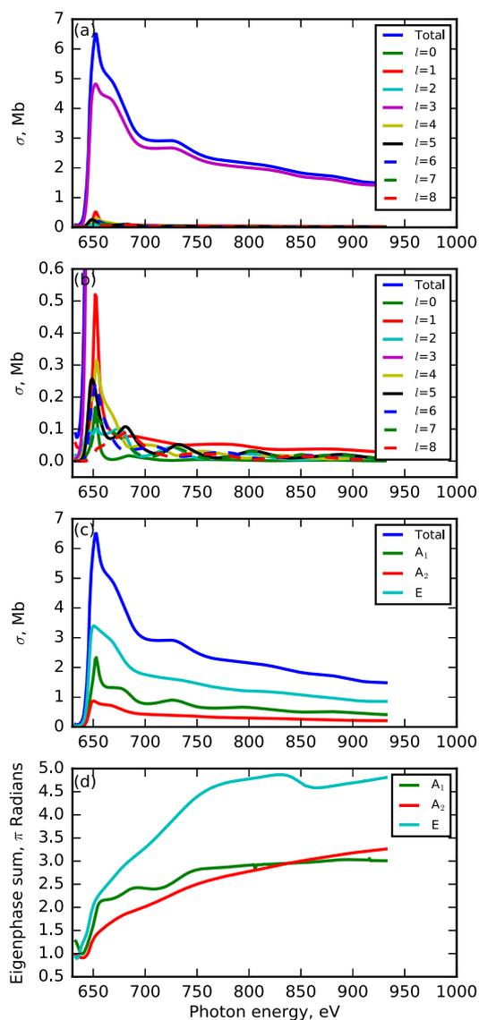
FIG. 4. (a) Photoionization cross section of the I  $3d$  level in  $\text{CH}_3\text{I}$ , calculated using the CMS- $X\alpha$  approach, decomposed into partial  $l$ -wave contributions, and expanded around the I atom. (b) Photoionization cross sections expanded to highlight the weaker  $l$ -wave contributions. (c) Photoionization cross sections decomposed into contributions made by symmetry adapted combinations of the angular basis functions. (d) The symmetry adapted eigenphase sums.
