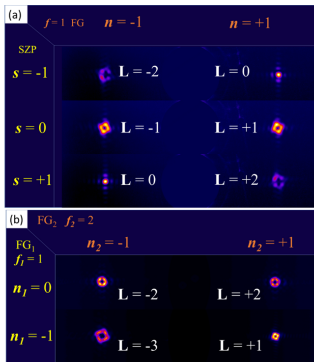
Figure 8 (a) Diffraction orders n = \pm 1 generated by the FG ( f = 1 ), illuminated using an SZP with s = -1 (top), s = 0 (middle) and s = +1 (bottom). (b) Intensity pattern obtained by aligning two fork gratings, \text{FG}_1 and \text{FG}_2 , in cascade: the first with f_1 = 1 and the second with f_2 = 2 . \text{FG}_2 is illuminated either by the zeroth order of \text{FG}_1 ( n_1 = 0 , top) or by its first negative order ( n_1 = -1 , bottom). The expected L values for each spot at the detector are indicated in white. The photon energy is 152 eV in all cases.
