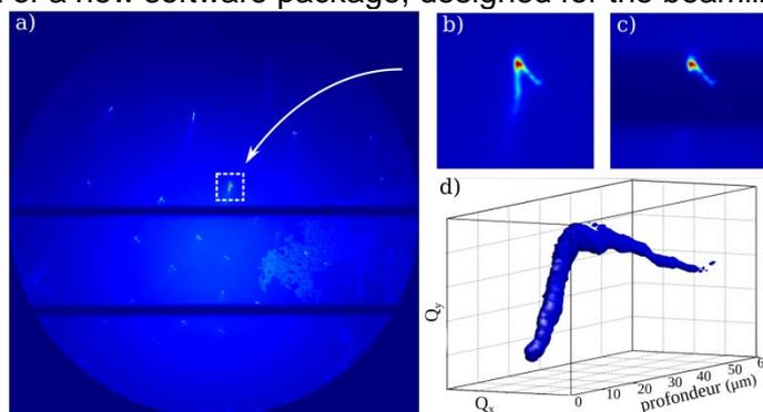
3D depth-resolved reconstruction of a diffraction spot: a) Laue pattern of a nitrided Ni-Ti alloy, using two tungsten wires of 50  $\mu\text{m}$  diameters, b) initial spot, c) spot partially masked by the wire d) isosurface representation of the reconstructed depth-resolved spot. The intensity spread directions provide information about the modes and heterogeneities of plastic deformation in the surface layer. (Sample: M. Fonovic, A. Leineweber, MPI, Stuttgart)
