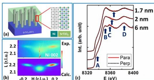
Figure: (a) Scheme of Ni NWs in SrTiO<sub>3</sub>. (b) XRD patterns: measured and calculated Ni 002 spot. (c) XANES parts of linear-dichroic XAS spectra with the x-ray polarization parallel (red solid lines) or perpendicular (black dashed lines) to the NWs: i) bulk-like Ni NWs of 6 nm diameter, with the characteristic Ni bulk peaks indicated by A, B, C and D arrows; ii) dichroic NWs of 2 nm diameter; iii) quasi-amorphous metallic Ni NWs of 1.7 nm diameter.
