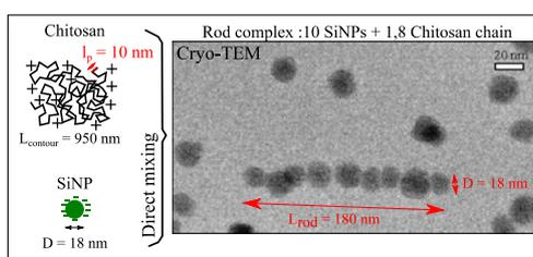
**Figure 1** Naïve representation of individual components (left) before complexation and cryo-TEM picture (right) of a stable nanorod complex obtained after mixing in water.
