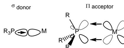
**Scheme 1.** The M-P bond as described by the DCD model.
