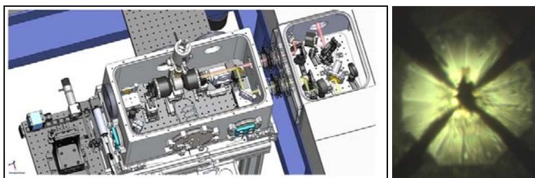
Fig. 1: Left panel: Schematic view of the high pressure – low temperature setup. Right panel: Optical microscope image of the sample with the four electrodes used to measure resistivity
