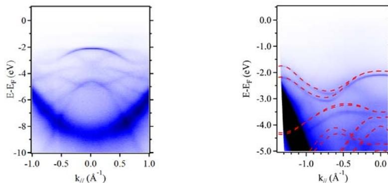
Figure 1:  $E$  vs  $k$  curves around  $\Gamma$  (left) and K (right) points in the first BZ of WS<sub>2</sub> ( $h\nu = 50$  eV). Red dotted lines are theoretical bands obtained with DFT calculations.
