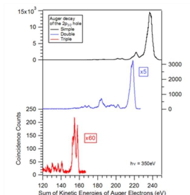
Figure 1. Auger spectra for the Auger decay of a K 2p hole by emission of one, two or three Auger electrons.
