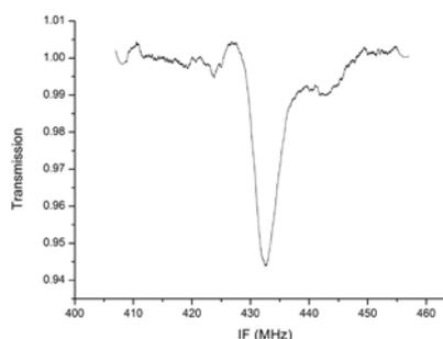
Fig. 2. Absorption line of D<sub>2</sub>O with sub-MHz resolution. LO frequency: 782.0388 GHz, T = 293 K, P = 50 μbar.
