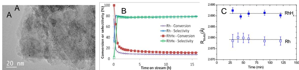
**Figure 1.** TEM image of 1.0 nm Rh-based nanocatalysts (A), conversion of butadiene and selectivity to butenes during the laboratory catalytic tests (B), time variation of nearest neighbor distance ( $R_{Rh-Rh}$ ) for Rh and RhH<sub>x</sub> catalysts, as obtained by EXAFS (C).
