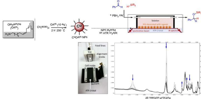
Figure 1 - Taylor-made ATR FT-IR cell, decorated with Cu NPs for reaction profiling
