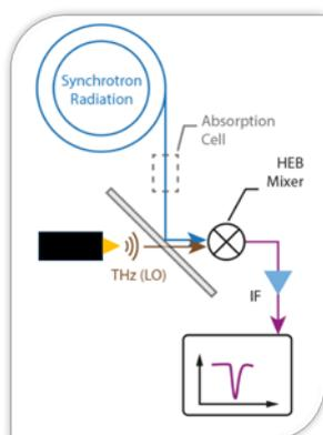
Fig. 1. Heterodyne detection scheme
