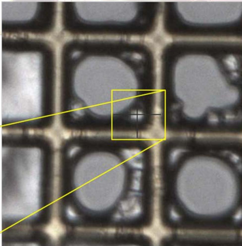
AcMNPV polyhedra crystals approx  $5 \times 5 \times 5 \mu\text{m}^3$  in size were mounted on a micromesh grid
