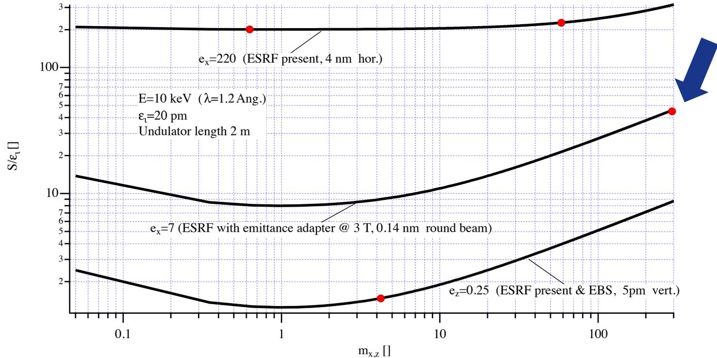
Beta matching requires too high solenoid field for round beam:  $B_s = \frac{\pi p_0}{eL\sqrt{r}}$  (easily > 100 T)
