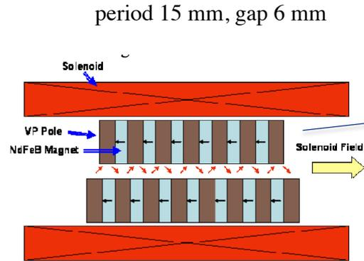
Figure 1: Schematic of a hybrid staggered undulator.
