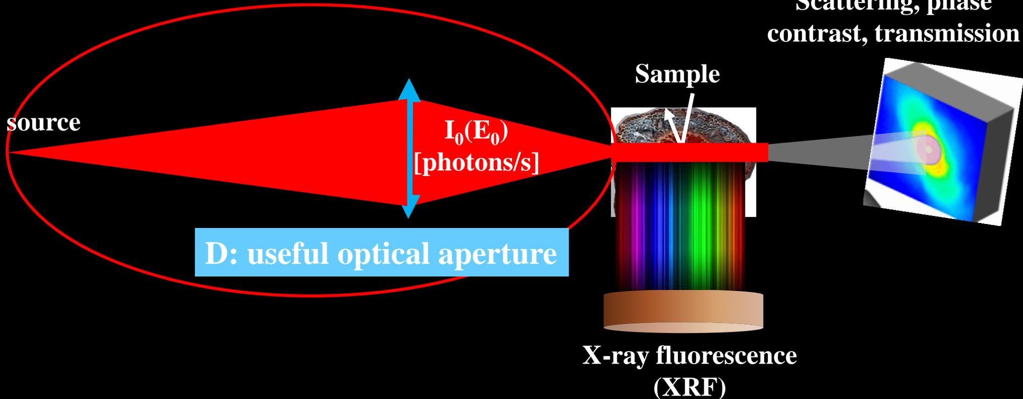
**Focused X-ray beam: intensity, size, focal depth, coherence properties influence the obtained image quality**
