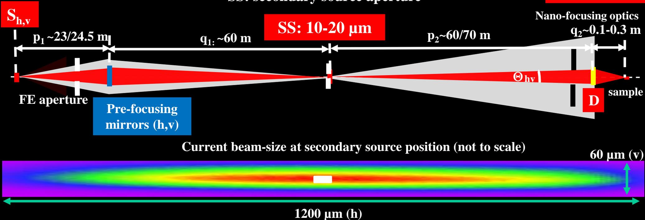
Coherent illumination is required to achieve optic-limited resolution ( $\sigma_{\text{DL}}$  diffraction limit)
