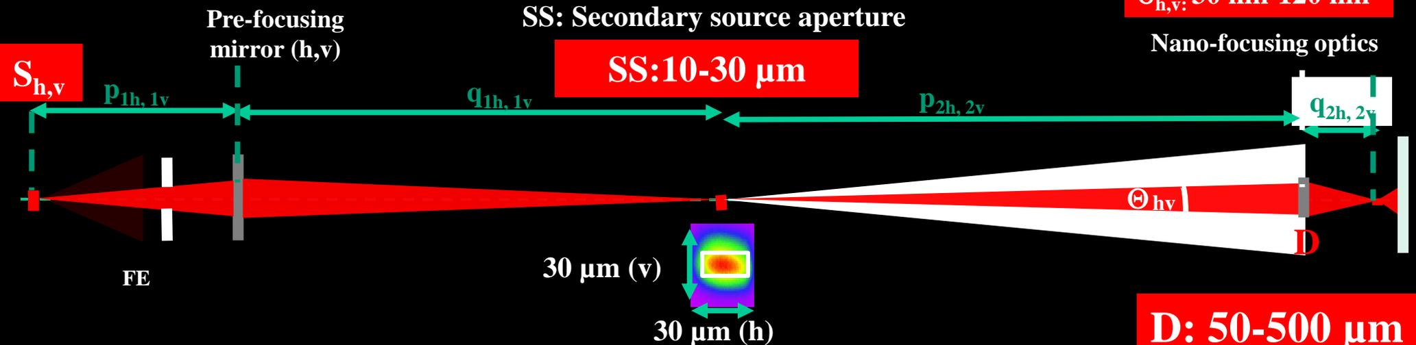
Beam at secondary source position (not to scale)
