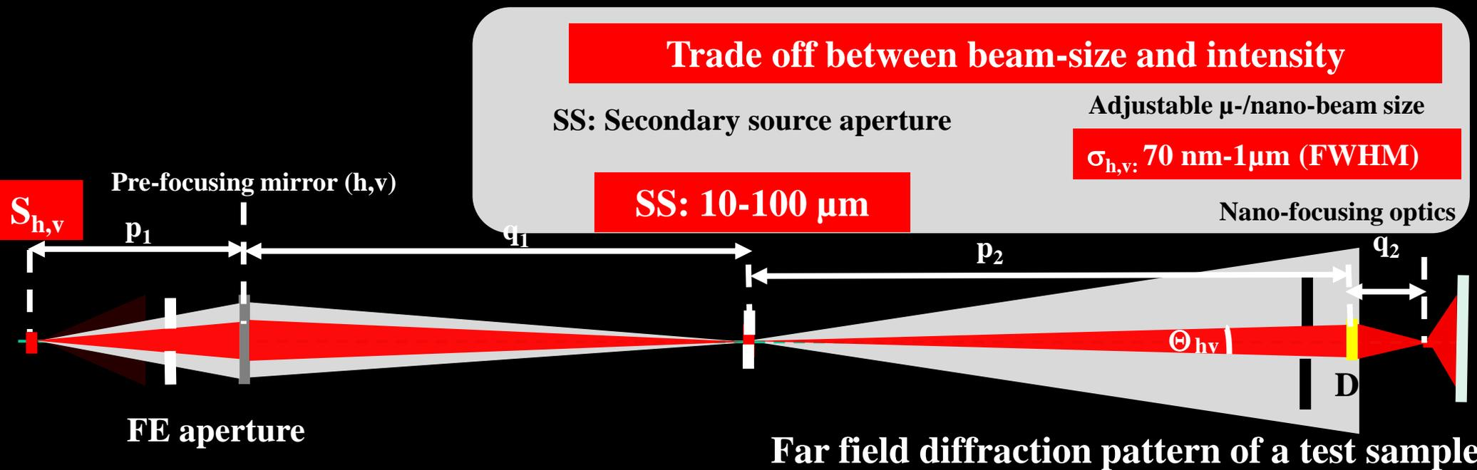
Coherent illumination (<1% of the beam intensity)
