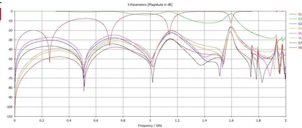
Coupling between electrodes
