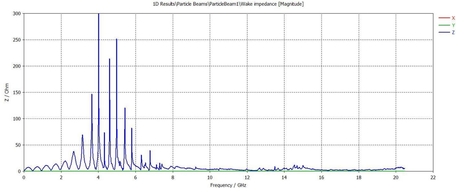
shows the real part of the longitudinal impedance, Impedance peaks are present between 3 and 6 GHz with high values which can disturb the beam.
