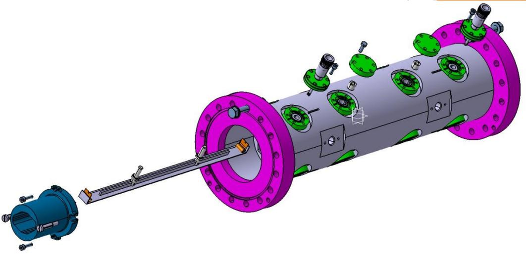
All parts are screwed together, so that the stripline can be fully dismounted for future needs.
