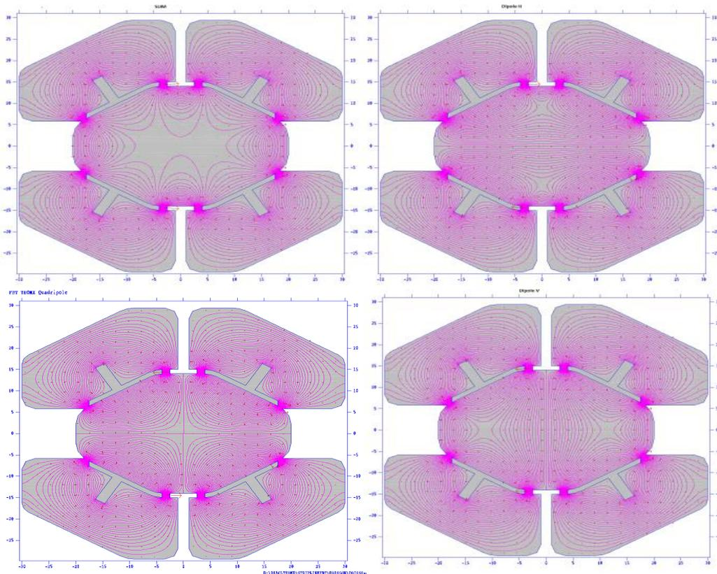
Poisson electromagnetics 2D software used to calculate the electric field for different dipole, quadrupole and sum mode
