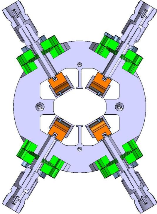
Feedthroughs are the standard CF flange N type adapted to our needs.
