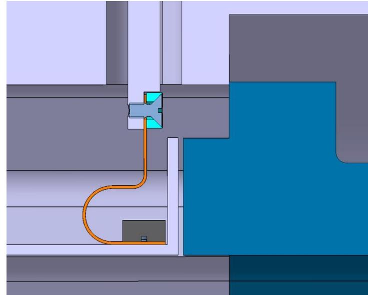
Electrical connections at both ends of the electrodes are made through a flexible copper sheet to avoid damage during baking process.
