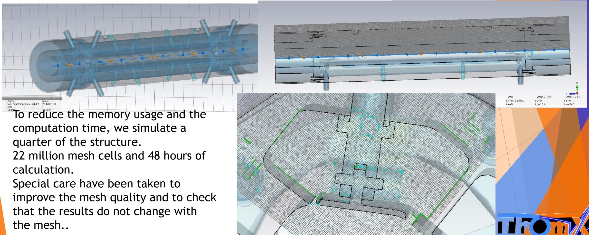
To reduce the memory usage and the computation time, we simulate a quarter of the structure. 22 million mesh cells and 48 hours of calculation. Special care have been taken to improve the mesh quality and to check that the results do not change with the mesh..
