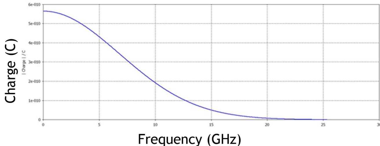
Charge distribution amplitude spectrum
