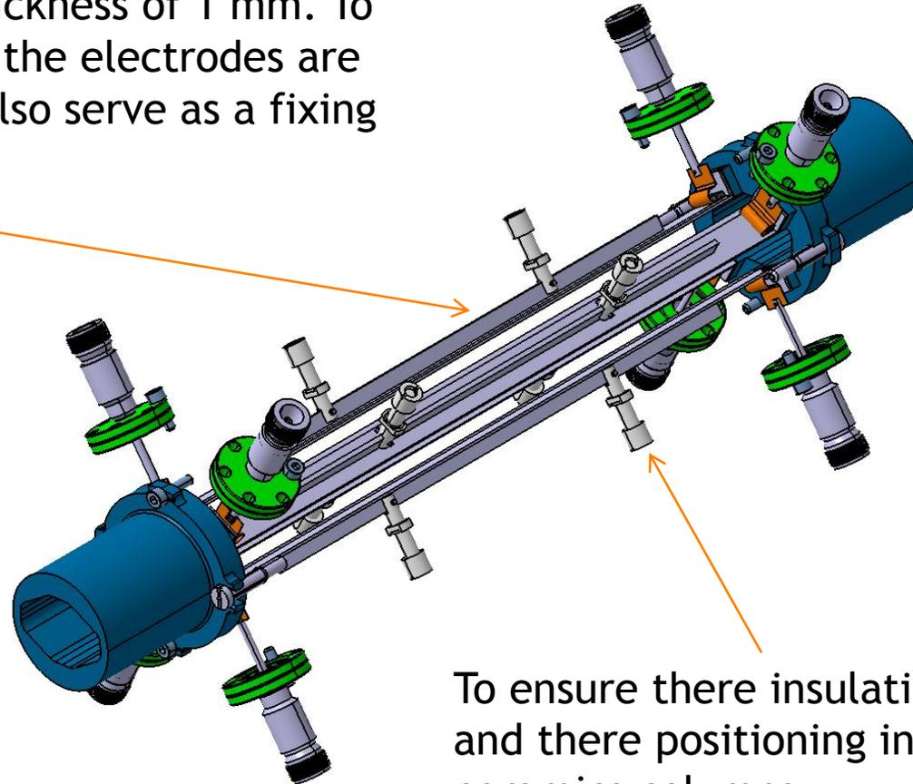
To ensure there insulation from the rest of the machine and there positioning inside the Chamber, it are taken by ceramics columns
