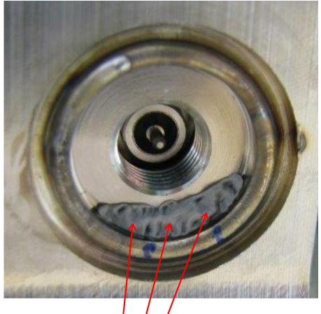
vacuum wax applied : the leak is stopped!
