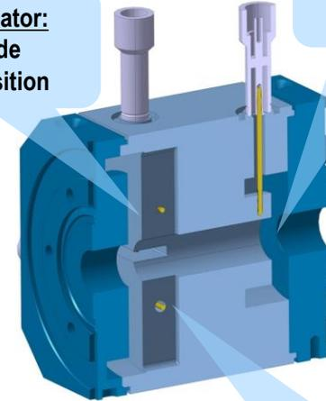
4 mode-selective waveguide couplers
