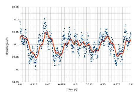
Moving Average Filter for Monochromator Position
