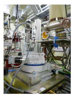
A motorised stage for multi-samples cell is available in replacement of the upper part of the multi-axis manipulator.
