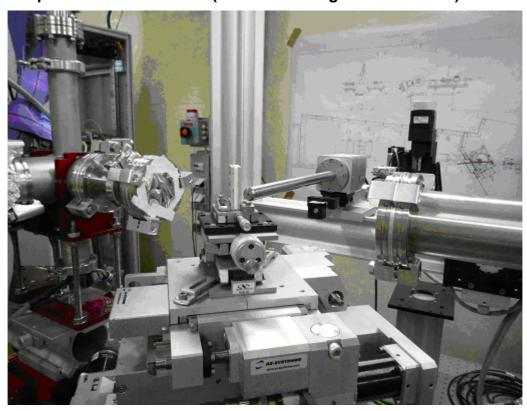
XRD set up (Image Plate MAR345 detector)
