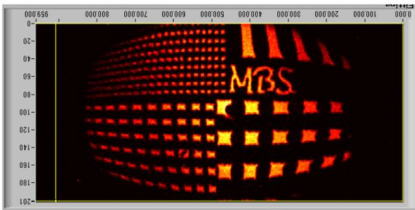
2D Angular mapping data taken by MBS A-1\_#0022 analyser with L3\_AS lens.
