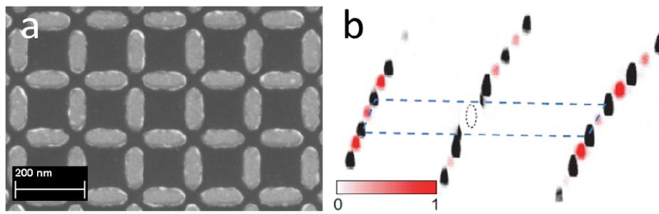
**Figure 1 :** a) Spin ice sample b) Experimental scattering pattern of Artificial Square Ice recorded at the Fe  $L_3$  edge (706.8 eV). The Bragg peaks highlighted in red are of pure magnetic origin and the black peaks are of combined structural/magnetic origin. Taken from [2]
