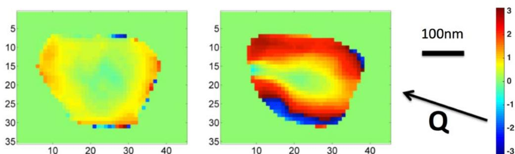
**Figure 1.** Phase image of the Au crystal before (left) and after (right) Fe deposition.
