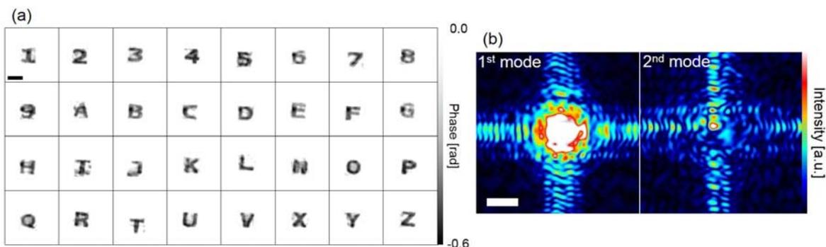
Figure 1 Reconstruction by multiple Fresnel CXDI. (a) Phase images of the thirty-two isolated objects. (b) Wavefront of the two independent probes. The scale bar is  $2 \mu\text{m}$ .
