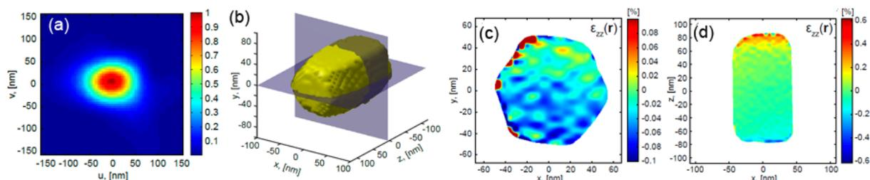
**Figure 1.** (a) Beam profile reconstructed by transmission ptychography; (b) Part of the nanowire in 3D reconstructed by Bragg CXDI; (c) and (d) 2D slices of strain distribution within the nanowire
