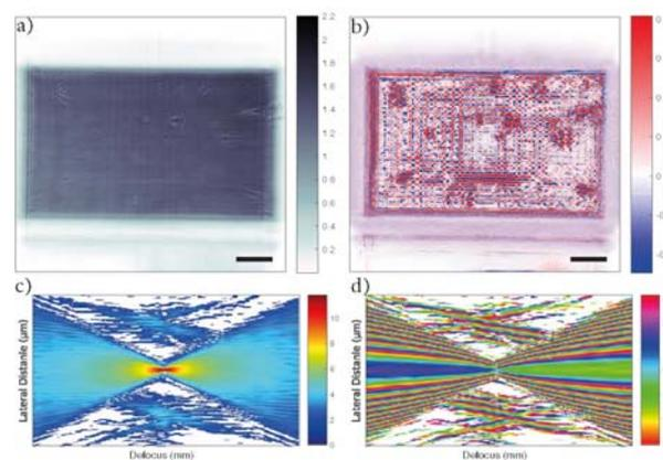
Fig. 1. Example for probe reconstruction using MMP. a) and b) show the recovered probe at the detector in amplitude and phase, respectively. c) and d) show a propagation profile in intensity and phase, respectively, around the focal plane for the vertical direction.
