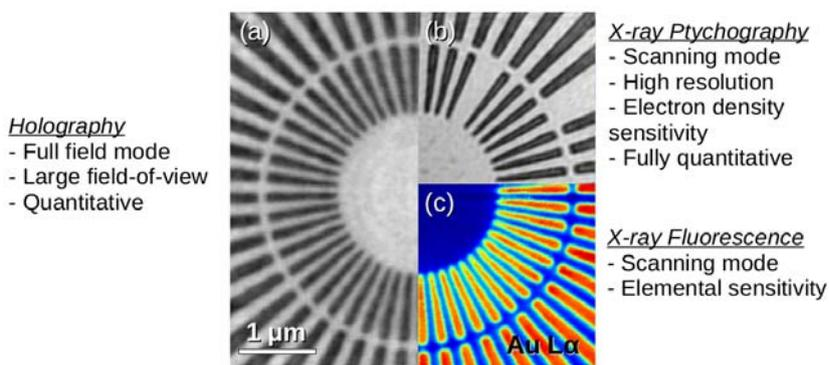
**Figure 1:** The techniques available at ID16A Nano-Imaging beamline, ESRF, applied to a 200 nm thick “Siemens Star” made of gold. (a) Holography. (b) Ptychography. (c) Fluorescence imaging.
