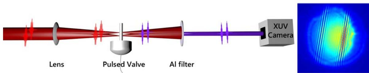
**Figure 1:** Schematic overview of the HHG setup. Two coherent infrared pulses produce HHG independently in a gas jet, and the resulting XUV pulse pair is detected with an XUV-sensitive CCD camera for interferometry and spectroscopy.
