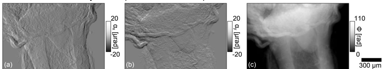
**Figure 1:** Refraction angle in horizontal (a) and vertical (b) direction and retrieved phase shift (c) of the bottom part of a small flower bud obtained with the proposed speckle acquisition and analysis method.
