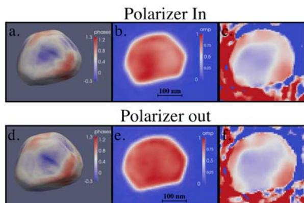
Figure 1: Top row: Gold nanocrystal reconstruction with the phase retarder in the beam showing (a) magnitude isosurface (25%) colored by phases (b) magnitude slice (c) phase slice. Bottom row: Reconstruction of same gold nanocrystal with the phase retarder out of the beam, showing (d) magnitude isosurface (25%) colored by phases (e) magnitude slice (f) phase slice.
