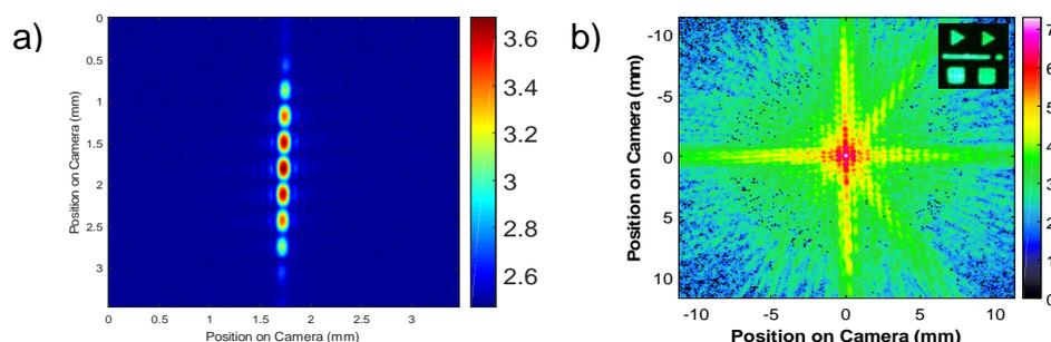
**Fig. 1.** (a) Diffraction from a double slit ( $1.5 \mu\text{m}$  separation) shows excellent contrast (log-scale). (b) Diffraction pattern from a sample with  $1 \mu\text{m}$  dimension ( $\text{NA}=0.7$ ). Inset shows a successful reconstruction of the object (log-scale).
