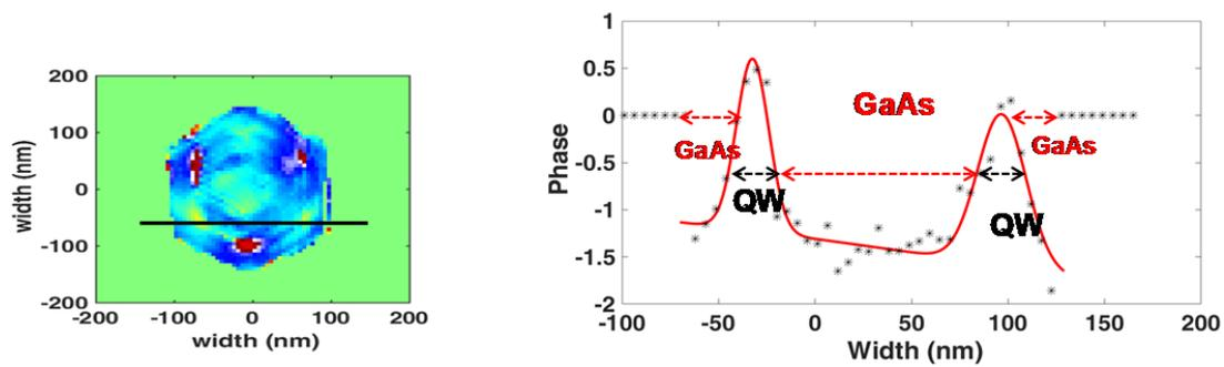
**Figure 2.** (left) Reconstructed phase in real space. (right) line cut along the corners of the nanowire showing the phase change at the expected position of InGaAs shell.
