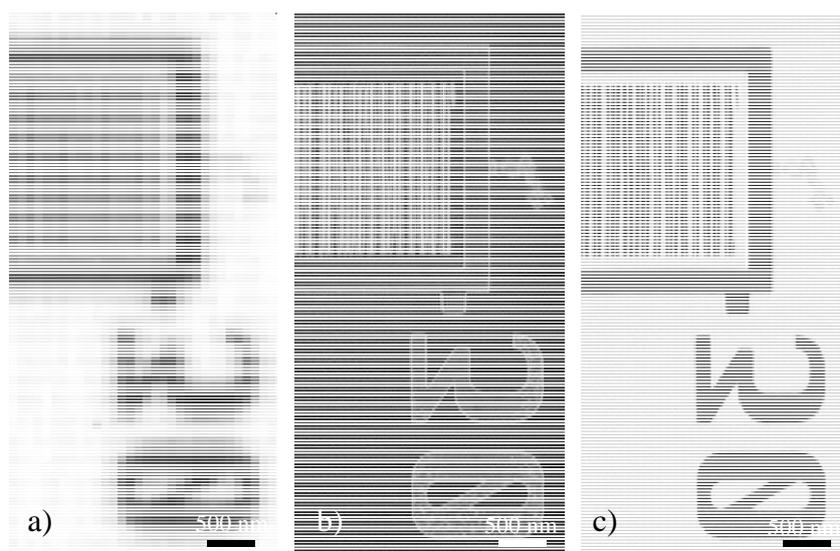
**Figure 1:** Resolution sample (Zeiss) with the smallest line size 30 nm imaged at energy 800 eV using high efficiency FZP with spatial resolution of 152 nm:
