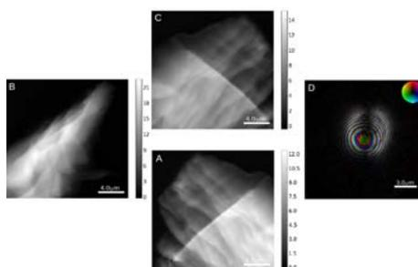
**figure 1:** A,B,C. shows the phase unwrapped projections of nanoporous gold sample at  $-90,0$  and  $90$  degrees respectively. The gray scale shows the phase shift in radians. D is the first mode of orthogonalized probe obtained from reconstructions.
