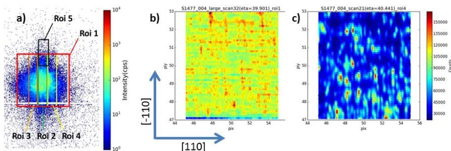
**Fig. 1** a) ROI definition b) ROI1 weak beam (-0.5°) 10x6μm<sup>2</sup> kmap on GaP(004). c) ROI4 strong beam kmap on GaP(004).
