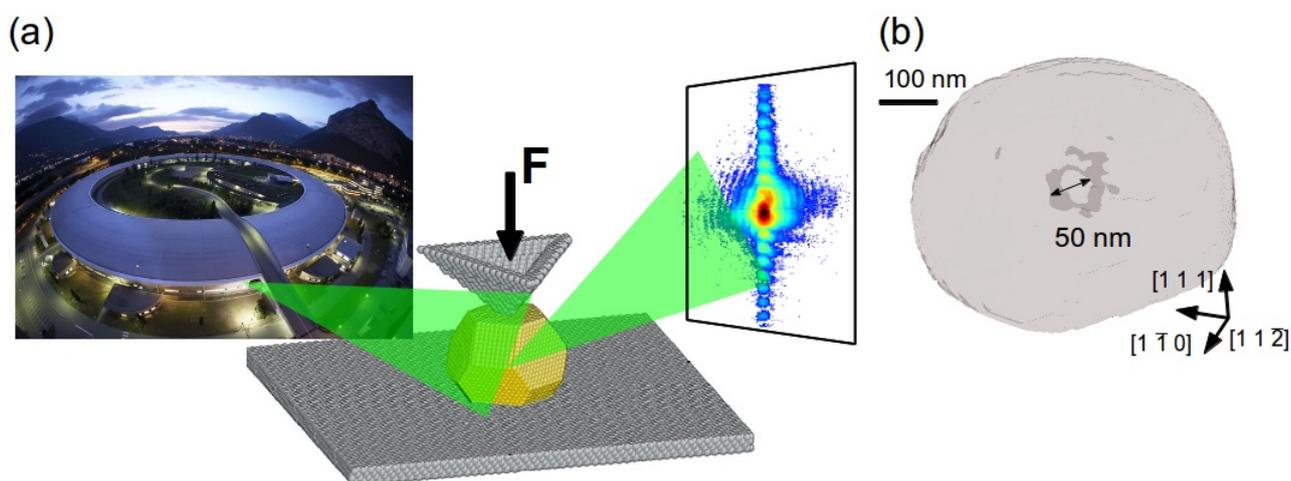
Fig. 1 (a) Schematics of the experiment and reconstructed electron density of the sample after indentation showing a prismatic loop trapped inside.
