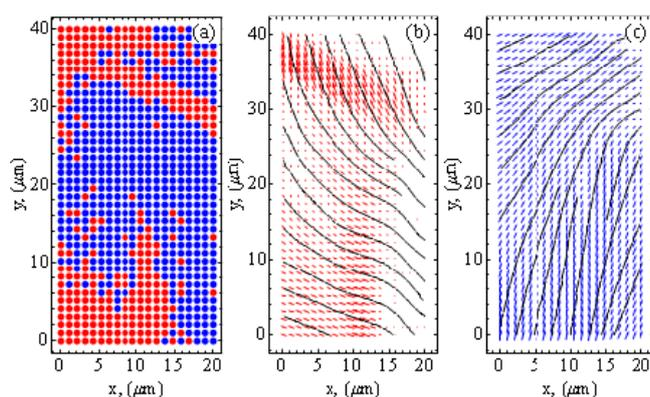
**Figure 1:** (a) Spatial distribution of distinct morphologies of crystalline poly(3-hexylthiophene) (P3HT) domains across the semicrystalline film, determined from the orientations of the (200) (b) and (020)/(002) (c) scattering peaks. Sample areas with predominant face-on (red points) and mixed (blue points) orientation of crystalline P3HT domains are visualized in (a).
