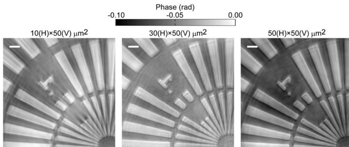
**Figure 1:** Phase images for the three slit openings reconstructed using the multiple-mode ePIE algorithm. The scale bar is 200 nm.
