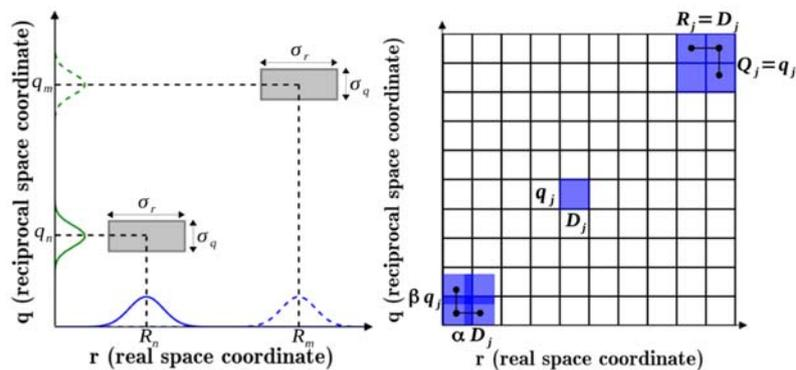
**Figure 1:** Representation of the ptychography phase-space. (left) The elementary signals as Heisenberg Boxes. (right) Phase-space coverage in critical and oversampling conditions. Figures from ref. [1].
