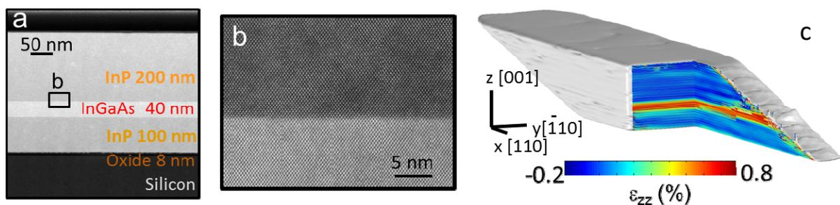
**Figure 1:** (a) Structure of the thin film on a scanning transmission electron microscopy image (high-angle annular dark field mode). (b) Zoom in on the top InP/InGaAs interface. (c) 3D Bragg ptychography strain result; the InGaAs layer is clearly evidenced, as well as some fluctuations inside the InP layers (the length of the black lines is 200 nm).
