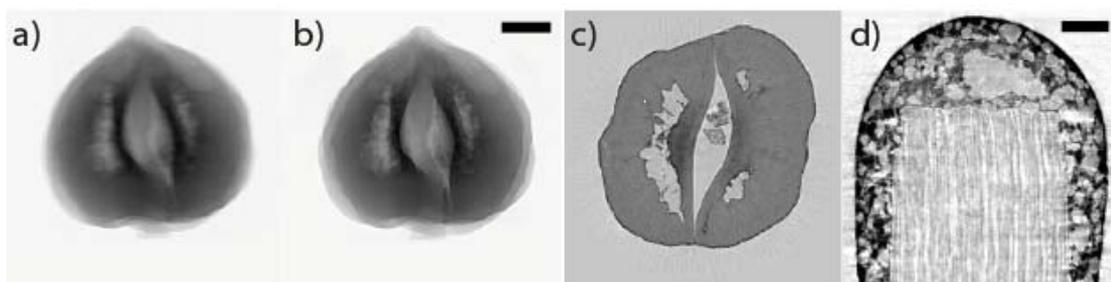
**Figure 1:** a) Acquired x-ray projection with an x-ray source spot of 1 x 0.1 mm (*horiz. x vert.*). The projection shows blurred side walls of the nut, while the top and bottom is sharply resolved. The reprojection (b) of the 3DRT-reconstructed nut shows high isotropic resolution. c) slice through the 3DRT-reconstructed nut. d) slice through a 3DRT-reconstructed match with Bronnikov-aided correction phase retrieval [2]. Scale bars: a)-c) 3 mm, d) 0.5 mm.
