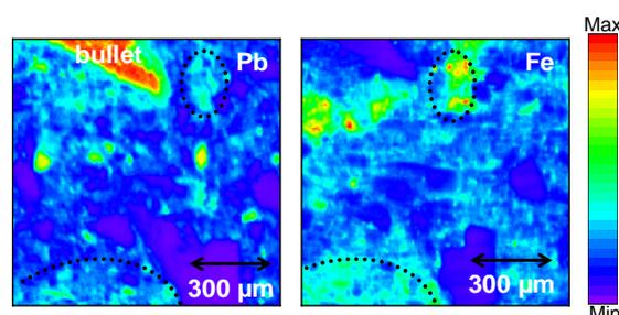
Fig. 1:  $\mu$ -XRF elemental map showing the correlation in Pb and Fe distribution in the soil located in the vicinity of a corroded bullet
