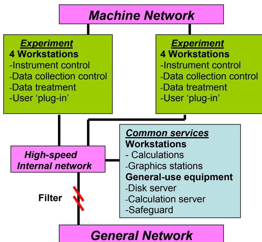
**Figure 2:** Proposed computing configuration for the first two experimental stations.
