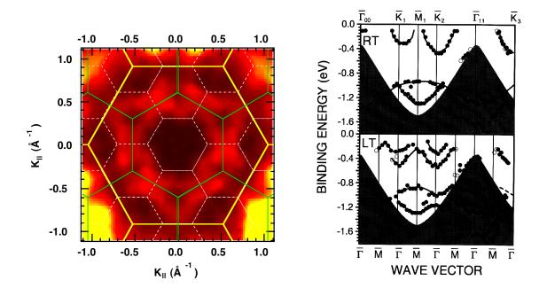
**Figure 8** (left panel) Fermi surface of  $(\sqrt{3}x\sqrt{3})R30^\circ$  reconstruction of Pb on Ge at RT and (right panel) experimental band structure of the same phase, PRB 57,14758(1998).
