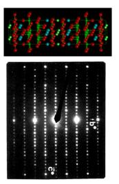
the prototypical systems in superconducting materials due to their crystal perfection. Figure 4. Structure and Diffraction pattern of a Bi2212 crystal. Those samples are
