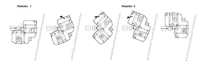
**Figure 12:** The scheme of the platform with the two end-stations is shown in the top part of the figure. The platform movement permitting the alternative positioning of Station I and II in line with the beamline is depicted in the bottom of the figure.
