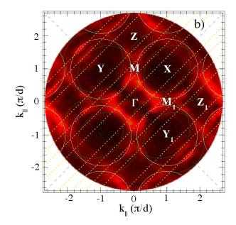
**Figure 5**. The figure shows large portions of the Fermi surface of a Fermi Surface of Bi<sub>2</sub>Sr<sub>2</sub>CaCuO<sub>8+ $\delta$ </sub> crystal at the optimum doping with Tc=91 K, (measured at the SU8, September 2000).
