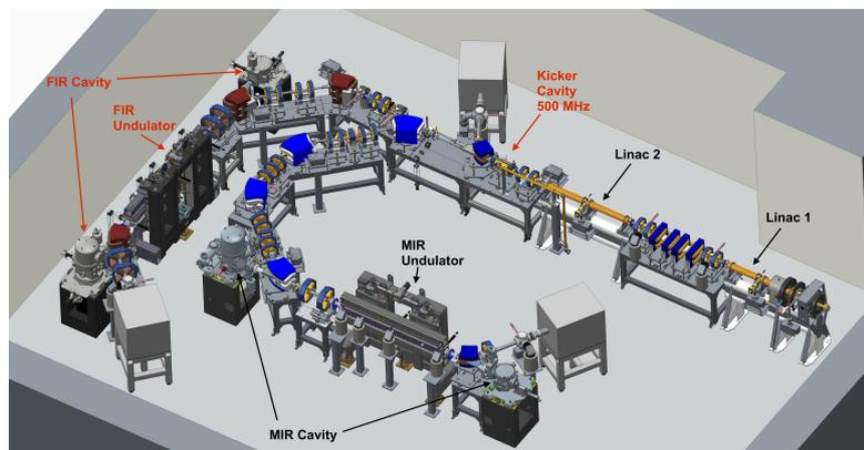
**Figure 1: Layout of the FHI FEL 2-color upgrade. A kicker cavity as well as the undulator, optical cavity, and electron beamline of the new FIR branch have been installed and commissioned in 2023.**
