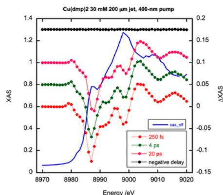
Fig. 1 pump-probe XAFS of  $\text{Cu}(\text{dmp})_2$  molecules using a liquid jet (diameter: 200  $\mu\text{m}$ )
