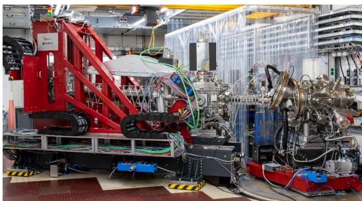
Fig. 1: hRIXS spectrometer and XRD chamber at SCS Instrument
