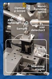
Scanning multi-length scale imaging with spatial resolution readily adaptable in the 100 nanometer - 1 micron range is provided routinely. This multilength scale "zoom-in" capability is well adapted to the study of complex heterogeneous samples and of tiny features embedded in intact mesoscale samples.
