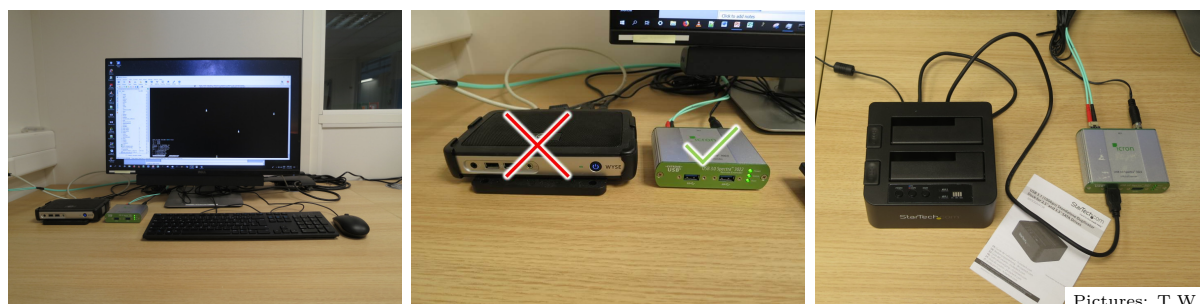
Figure 5.5: Facilities for retrieving data. Left: One of the 3 data PC consoles in the ANATOMIX meeting & data room. Center: USB extenders on a console. The black box on the left is a USB-2 extender, not suited for data transfer to your hard disks because it is too slow. The smaller green box is the USB-3.0 extender for data transfer. Right: Dock for SATA disks, an alternative to USB disks.
