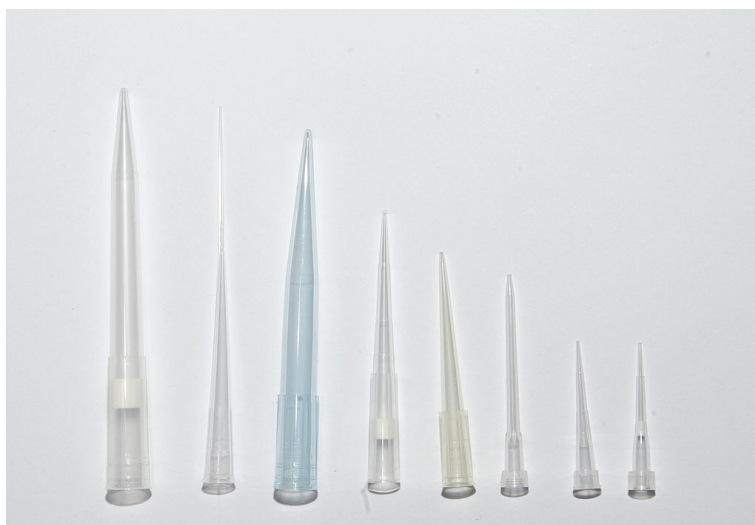
Figure 4.8: Pipette tips can be suitable containers for smaller samples in liquid.
