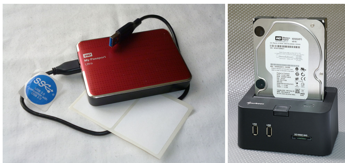
Figure 4.10: External hard disk remain the preferred way of transferring tomography data from ANATOMIX to users’ home laboratories. Left: USB 3.0 disk with flat USB-A connector. Right: SATA disk in docking station (docking stations are available at the beamline).
