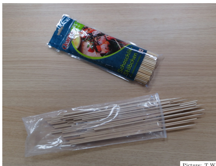
Figure 4.5: Wooden shashlik sticks from the grocery store, such as those shown in this picture, can be used as an alternative to metal sample pins or SEM stubs. Make sure they have a diameter of 3 mm so they fit snugly into the goniometer head.
