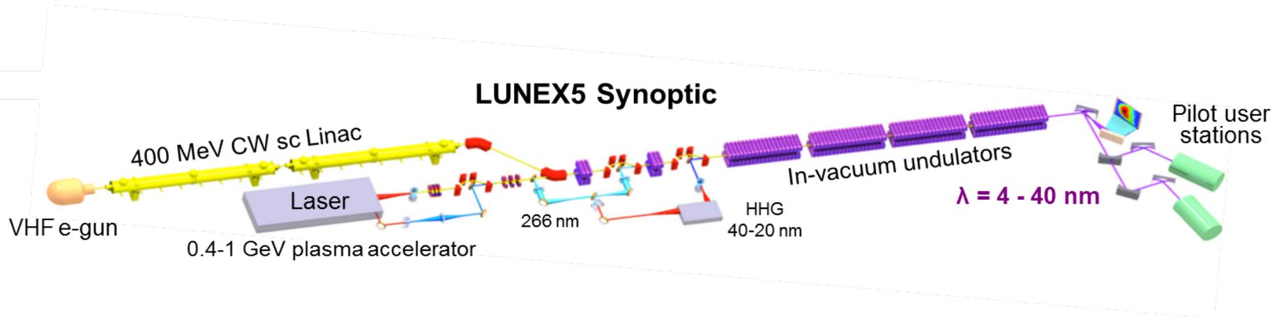
**Phase 1 : based on a 400 MeV CW sc Linac → explore advanced FEL techniques and applications**
