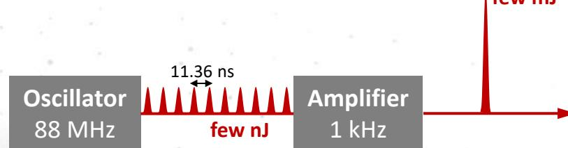
**Chirped pulse amplification**
