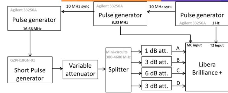
Test bench for acceptance test
