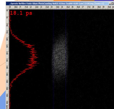
*Cerenkov radiation longitudinal measurement on PHIL with ThomX streak camera (photon counting mode)*
