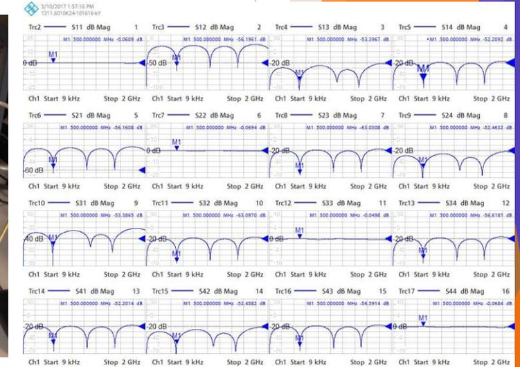
*Calibration based on “Lambertson” method using a logic network analyzer*
