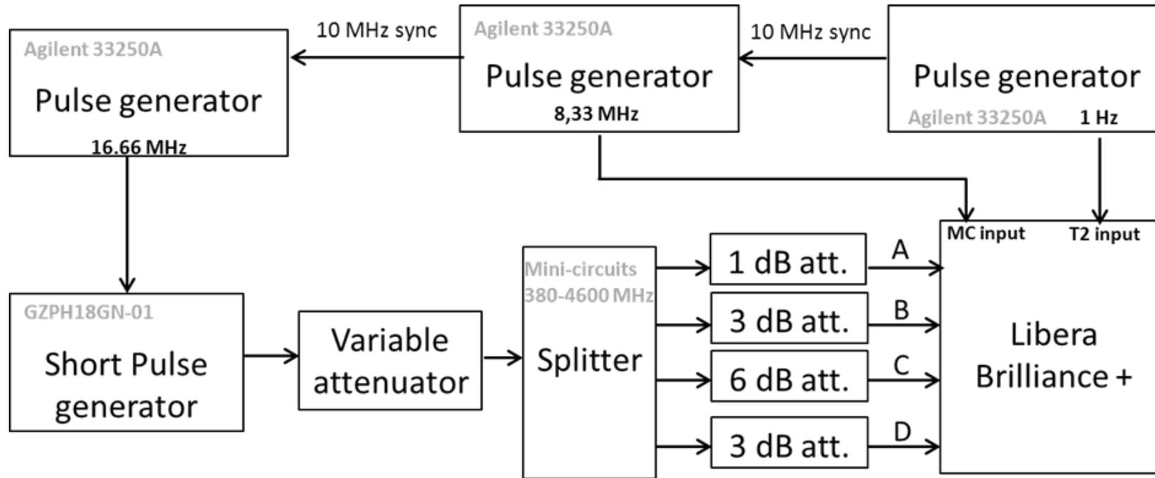
*Test bench for acceptance test*
