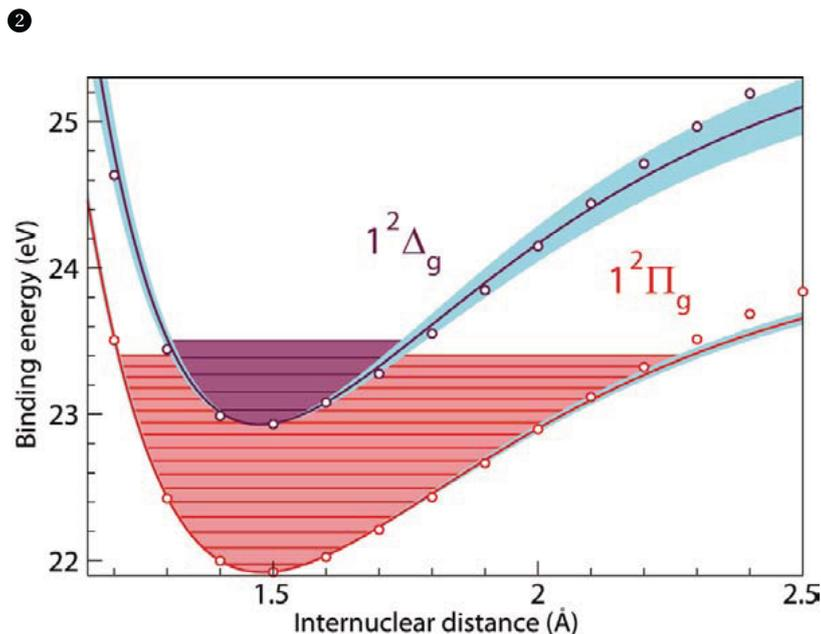
**Figure 2: Comparison between the reconstructed molecular potentials based on ultrahigh resolution RPE data and ab initio calculated potentials (open circles). The error bars are shown as blue colored areas.**
