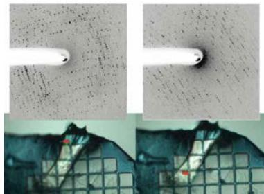
Two X-ray diffraction images taken from an "ugly" crystal on PROXIMA 2: On the left, a zone at the top of the crystal was exposed, and the diffraction pattern is messy with spots at irregular spacings. On the right, a zone at the bottom of the crystal was exposed, and the diffraction pattern is clean with spots at regular spacings. The red rectangle marks the position and size of the X-ray beam. The sample is mounted on a plastic support with a 25 micron mesh.
