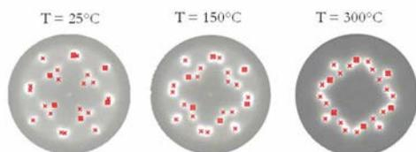
Figure 2 : Pole figures measured *in situ* for a  $\text{Pd}_2\text{Si}$  film on  $\text{Si}(001)$  around the  $111\text{Pd}_2\text{Si}$  reflection at different temperatures.
