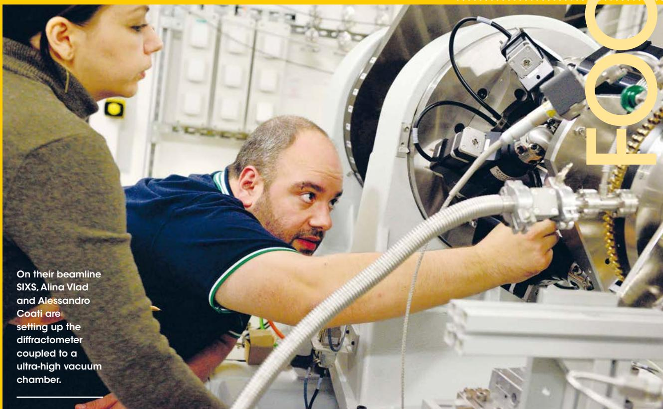
On their beamline SIXS, Alina Vlad and Alessandro Coafi are setting up the diffractometer coupled to a ultra-high vacuum chamber.
