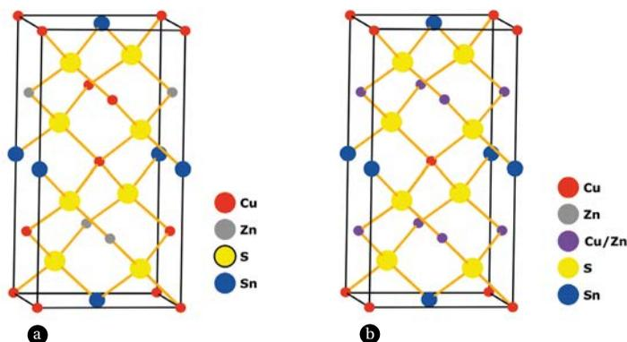
Figure 2 : Kesterite-type structure of  $\text{Cu}_2\text{ZnSnS}_4$ , a) ordered (space group  $I\bar{4}$ ) or b) disordered (space group  $I4_2m$ )
