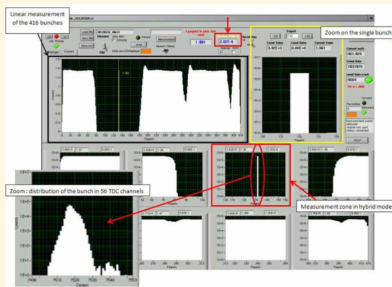
figure 2 : Purity measurement application in the control room.
