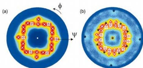
Figure 1 : (a)-(b) Pole figures measured for a  $\text{Pd}_2\text{Si}$  film on  $\text{Si}(001)$  around  $111\text{Pd}_2\text{Si}$  and  $212\text{Pd}_2\text{Si}$  reflections.  $0^\circ \leq \phi \leq 360^\circ$  and  $2^\circ \leq \psi \leq 88^\circ$ . The white crosses (black diamonds) show the simulated position of the  $\text{Pd}_2\text{Si}$  film peaks (substrate).
