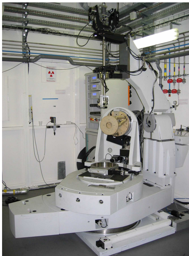
Figure 2: Diffractometer design by E. Newport-Microcontrol Inc. (X95 basis) at ESRF BM26 beamline.
