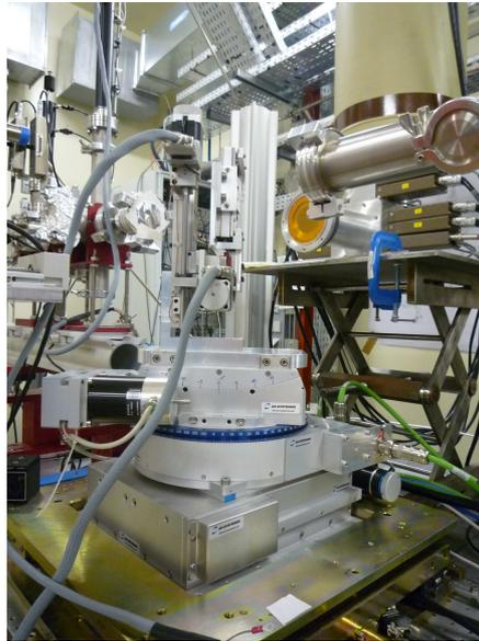
A motorised stage for multi-samples cell is available in replacement of the upper part of the multi-axis manipulator.
