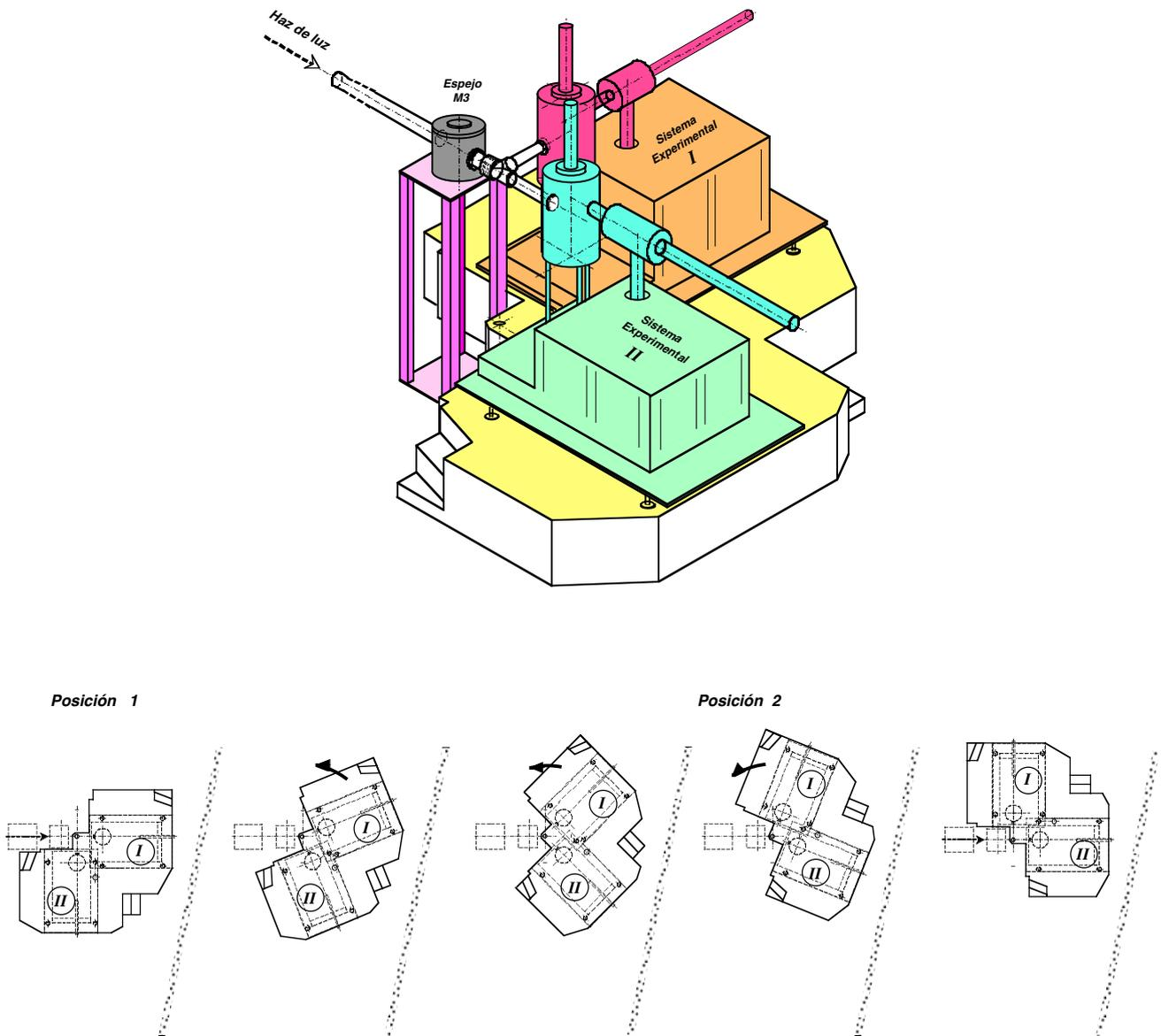
**Figure 12:** The scheme of the platform with the two end-stations is shown in the top part of the figure. The platform movement permitting the alternative positioning of Station I and II in line with the beamline is depicted in the bottom of the figure.
