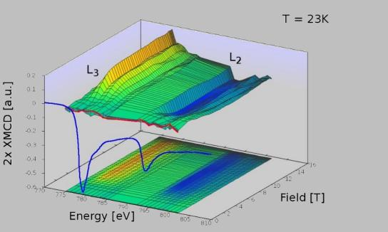
XMCD and XAS at the Co  $L_{2,3}$  edges measured in transmission for a 30 nm film of Co(S<sub>0.88</sub>Se<sub>0.12</sub>)<sub>2</sub>. The expected transition at ~4 T is clearly evidenced.
