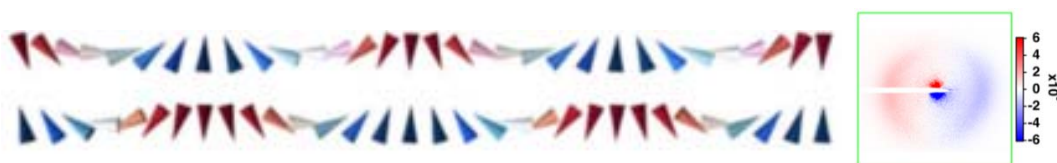
Figure 1 : (Left) Cross section of a calculated magnetic configuration of spin spirals antiferromagnetically coupled in a bilayer (from W. Legrand et al. Nat. Mater. 19 , 34 (2020))
