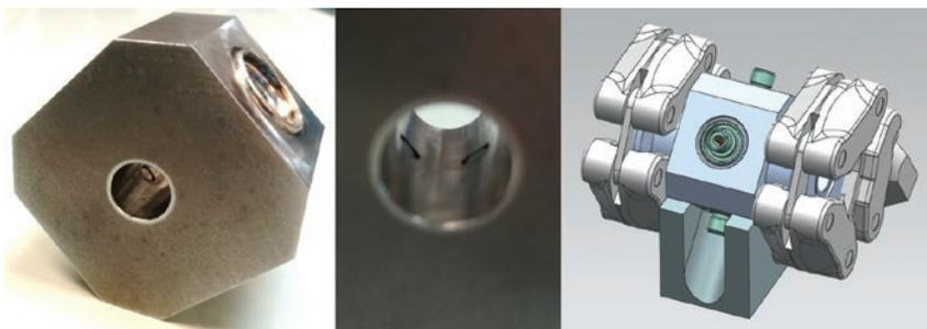
Figure 86: BPM first prototype with 3 mm diameter buttons on a 10 mm diameter block (left), inside view (center), support (right)
