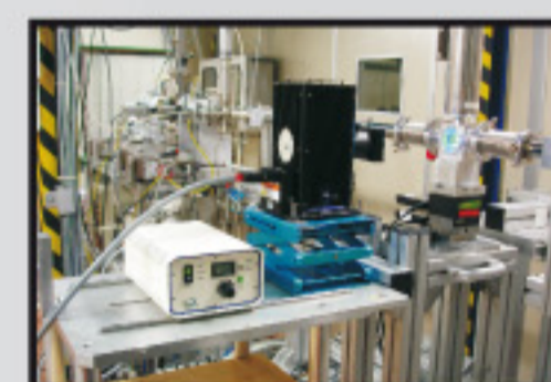
80K (-193°C) setup for light induced electron transfer measurements (XAFS beamline, Elettra synchrotron Italy).
