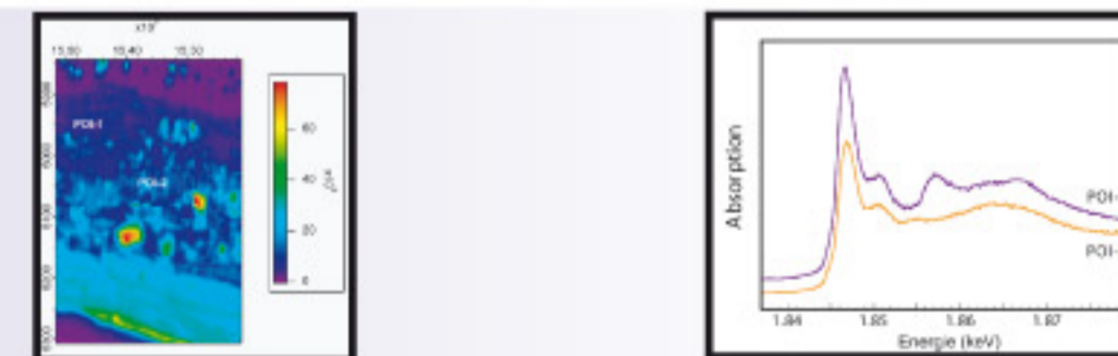
Silicon (Si) mapping and speciation to characterise silicate minerals present in a mineral crust (Joeri valley, Switzerland).
