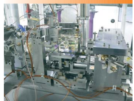
Figure 2: The spectrometer installed on the DESIRS beamline. The 'interferometer' part is visible in the middle (mirrors).
