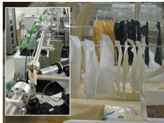
Samples and experimental setup. on the left: experimental setup (DIFFABS- SOLEIL) on the right: general view of prepared samples © CRCC
