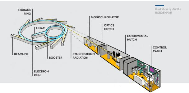
Along their path in this ring imposed by magnetic fields, the electrons lose some of their energy in the form of light radiation, or photons. With every turn, this extremely bright light is emitted, over a range of wavelengths from infrared to X-rays, and covering visible and ultraviolet light. To produce even more intense beams of light, the electrons also pass through specific magnetic devices that make their trajectory undulate.
