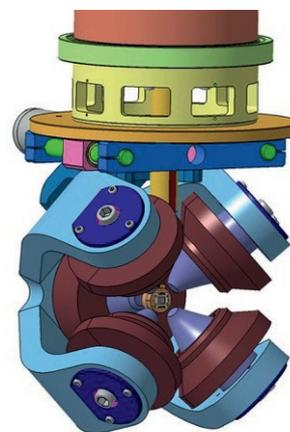
Figure 2: SOLEIL prototype of a complex 5 coils magnetic system to apply 3D magnetic fields at the sample position while keeping the scattering space free
